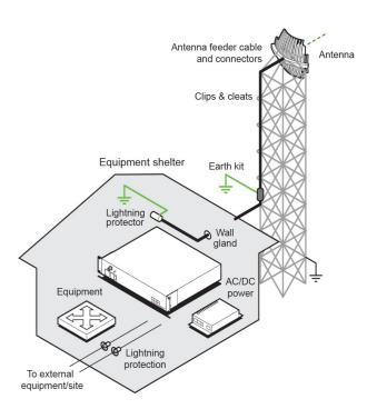
Connect the flexible coaxial jumper cable between the lightning protector and radio antenna connector.
