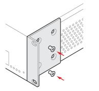
Connect the radio terminal's earth stud to the rack with the Earth cable using the 8 mm spanner
