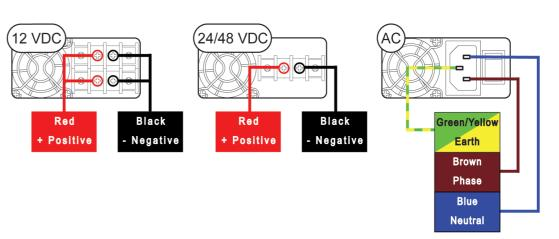
For DC power supplies, switch on the external power supply.For AC power supplies, turn the radio power switch on.
